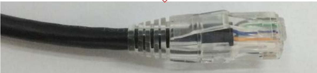
**Step 6:** Use the crimp tool to press the plug and the hook connector
